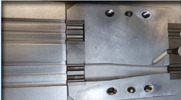
One cavity mold - Horizontal Injection
