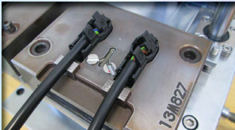
Two cavities mold - Vertical Injection
