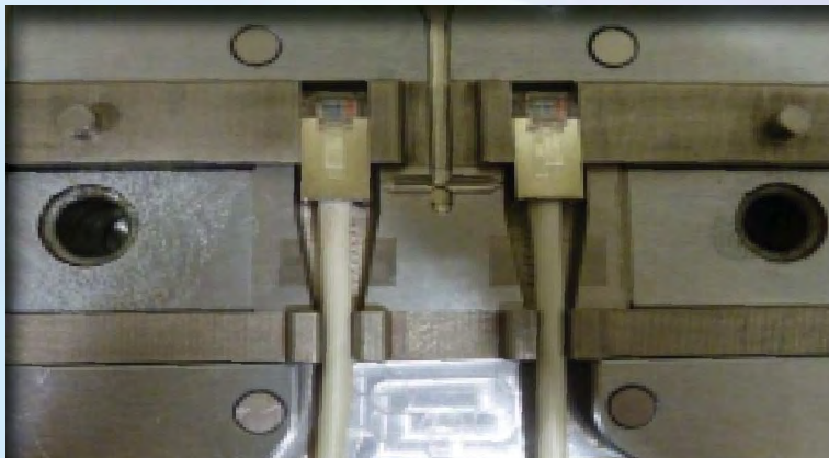
Two cavities mold - Horizontal Injection
