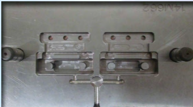
Two cavities mold - Horizontal Injection
