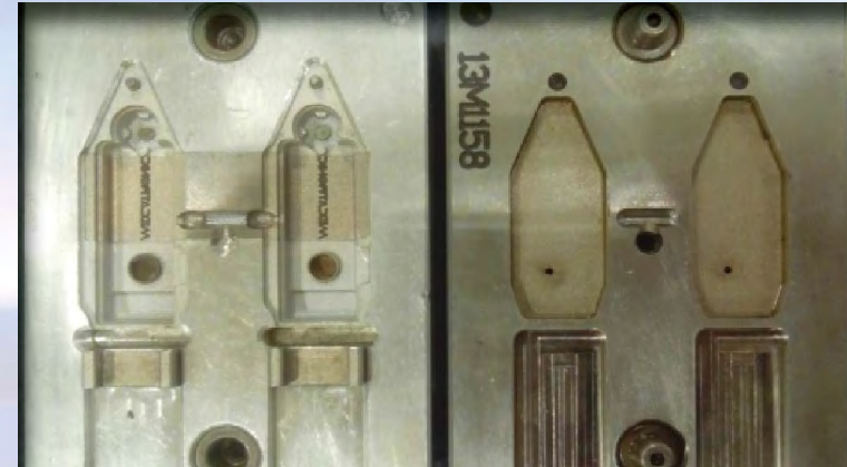
Mold 2 - Two cavities, Vertical Injection Final Shot
