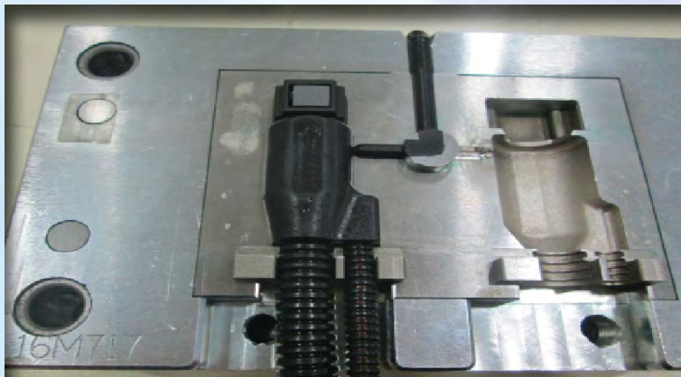
Two cavities mold - Horizontal Injection
