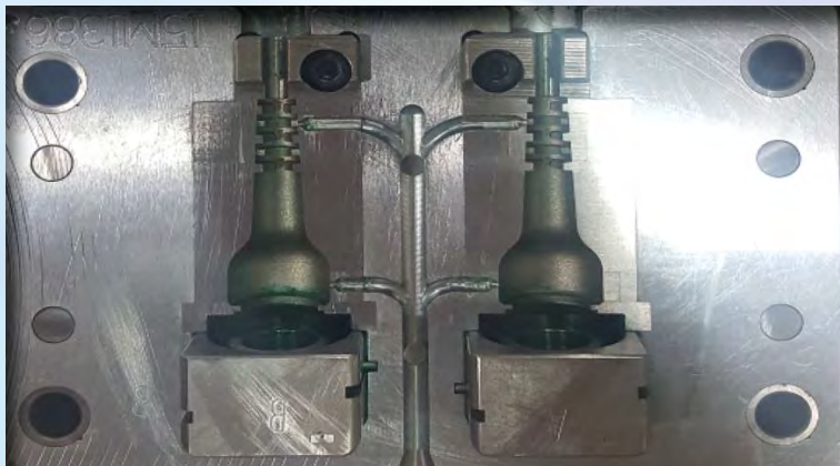
Two cavities mold - Horizontal Injection
