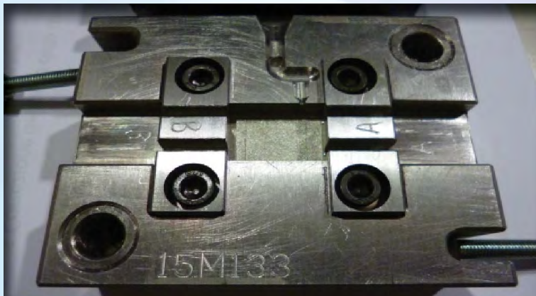
One cavity mold - Horizontal Injection
